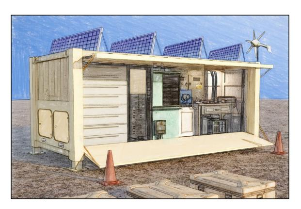
The MC3 Cube or multiple MC3 Cubes can be provided with a stand-alone utility module that can support several clinical modules with all utility needs using sustainable and low decibel/insulated technologies. These technologies may include PV Solar, Wind accessory, heat pump, ECM motors, and Micro turbine. Unlike other potential additives, Clean Cubes will not require any power support from an existing FOB power supply or local infrastructure.
